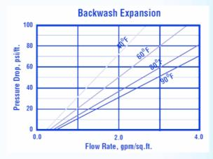
**Backwash:** After each cycle the resin bed should be backwashed at a rate that expands the bed 50 to 75 percent. That will remove any foreign matter and reclassify the bed.
